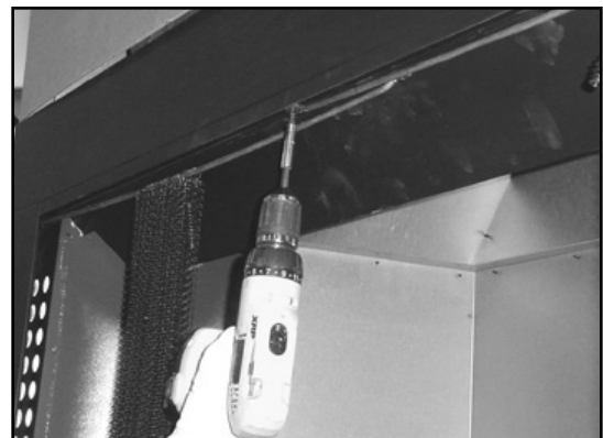
Figure 4.8 Removing the Screen Rods
